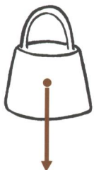
Figure 5. The centre of gravity is a point at the exact centre of a body's mass. A rigid object behaves as if gravitational pull concentrate all its force at this point.
