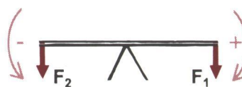
Figure 4. The force F_1 has a clockwise turning effect on the board. Such a moment is usually said to be positive. The turning effect of F_2 is directed counter-clockwise and, correspondingly, the moment is said to be negative.
