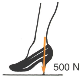
Figure 12. .... while a 50-kg woman in spike heels at heel strike exerts a pressure which is 5 MPa, i.e. 25 times greater!
